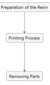
The material should be processed at room temperature. Before usage the material should be shaken well. Pour it slowly in the vat and wait a couple minutes, until smooth, bubble-free surface is obtained before starting the print job.
