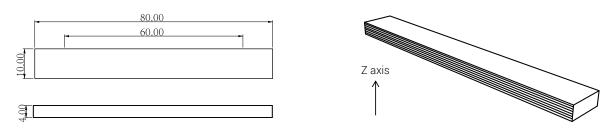
Fig 2. Flexural testing specimen
