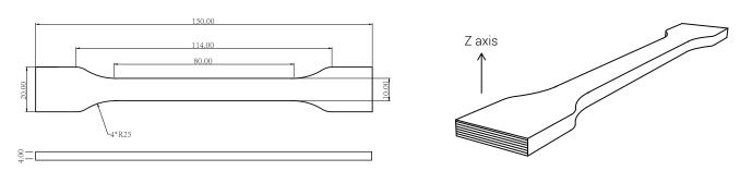
Fig 1. Tensile testing specimen
