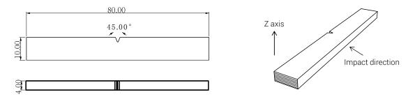
Fig 3. Impact testing specimen
